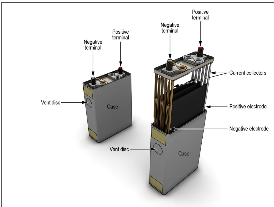
**Figure 3.** Cell design with three internal electrode winding assemblies.
