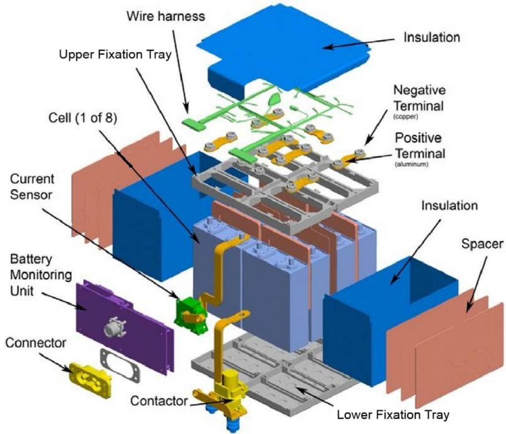
**Figure 2.** Components of the main or APU battery.
